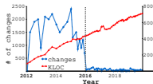
Figure 1. Rust History. (Each blue point shows the number of feature changes in one release version. Each red point shows total LOC in one release version.)
